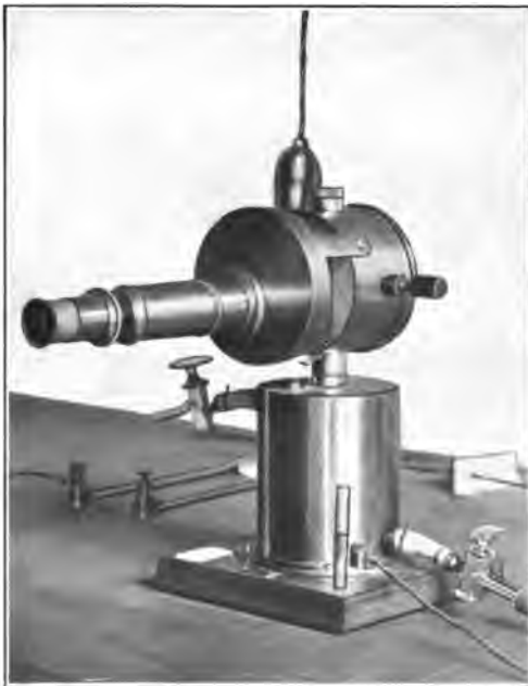
B. ELECTROSCOPE WITH INTERCHANGEABLE IONIZATION CHAMBER. THE ELECTRIC LIGHT SOCKET AND WIRE ABOVE THE INSTRUMENT ARE NOT PART OF IT.
